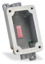
Killark device/splice box, feed through, (1) gang, factory sealed, (2) 3/4in female NPT conduit entries, aluminum. Use with FXCS series factory sealed cover assemblies for hazardous locations.
