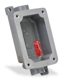
Killark device/splice box, feed through, (1) gang, factory sealed, (2) 1/2in female NPT conduit entries, aluminum. Use with FXCS series factory sealed cover assemblies for hazardous locations.
