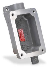
Killark device/splice box, dead end, (1) gang, factory sealed, (1) 1in female NPT conduit entries, aluminum. Use with FXCS series factory sealed cover assemblies for hazardous locations.
