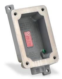
Killark device/splice box, dead end, (1) gang, factory sealed, (1) 3/4in female NPT conduit entries, aluminum. Use with FXCS series factory sealed cover assemblies for hazardous locations.
