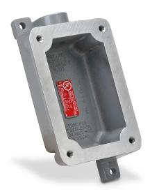
Killark device/splice box, dead end, (1) gang, factory sealed, (1) 1/2in female NPT conduit entries, aluminum. Use with FXCS series factory sealed cover assemblies for hazardous locations.
