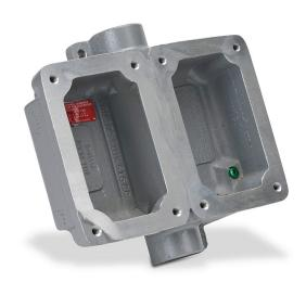
Killark device/splice box, feed through, (2) gang, factory sealed, (2) 1in female NPT conduit entries, aluminum. Use with FXCS series factory sealed cover assemblies for hazardous locations.
