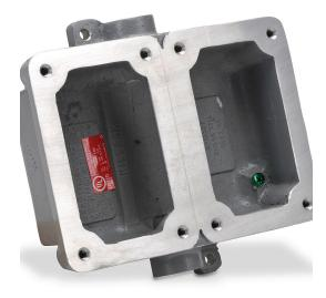
Killark device/splice box, feed through, (2) gang, factory sealed, (2) 3/4in female NPT conduit entries, aluminum. Use with FXCS series factory sealed cover assemblies for hazardous locations.
