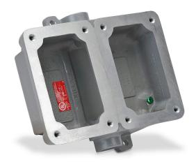
Killark device/splice box, feed through, (2) gang, factory sealed, (2) 1/2in female NPT conduit entries, aluminum. Use with FXCS series factory sealed cover assemblies for hazardous locations.
