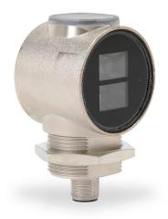
Photoelectric sensor, rectangular, polarized retroreflective, visible red light emission, 0.1-1.5m sensing distance, light-on, PNP, 3-wire, 4-pin M12 quick-disconnect.
