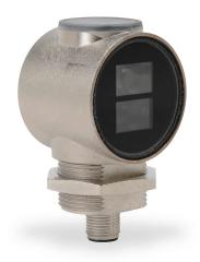
Photoelectric sensor, rectangular, polarized retroreflective, visible red light emission, 0.1-1.5m sensing distance, dark-on, PNP, 3-wire, 4-pin M12 quick-disconnect.
