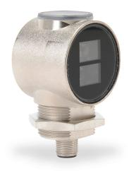
Photoelectric sensor, rectangular, polarized retroreflective, visible red light emission, 0.1-1.5m sensing distance, dark-on, NPN, 3-wire, 4-pin M12 quick-disconnect.
