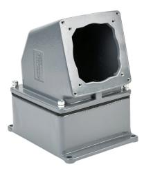
Bryant four-way back box, (1) 1-1/2in female NPT conduit entries, cast aluminum housing, gray. For use with Bryant 60A and 100A devices. Requires AP60 adapter plate for 60A devices or AP100 adapter plate for 100A devices.
