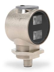
Photoelectric sensor, rectangular, diffuse with background suppression, visible red light emission, 50-800mm sensing distance, light-on, PNP, adjustable, 300 Hz switching frequency, metal housing, 4-pin M12 quick-disconnect.
