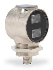
Photoelectric sensor, rectangular, diffuse with background suppression, visible red light emission, 0-600mm sensing distance, light-on, NPN, 3-wire, 4-pin M12 quick-disconnect.
