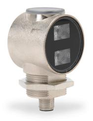
Photoelectric sensor, rectangular, diffuse with background suppression, visible red light emission, 0-600mm sensing distance, light-on, NPN, 300 Hz switching frequency, metal housing, 4-pin M12 quick-disconnect.
