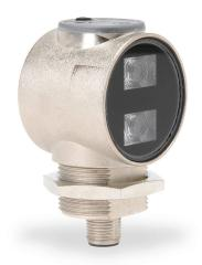
Photoelectric sensor, rectangular, diffuse with background suppression, visible red light emission, 50-800mm sensing distance, light-on, NPN, adjustable, 300 Hz switching frequency, metal housing, 4-pin M12 quick-disconnect.
