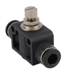
NITRA pneumatic push-to-connect fitting, inline flow control valve, thermoplastic (PBT) body, (1) 1/4in push-to-connect to (1) 1/4in push-to-connect. Package of 2.
