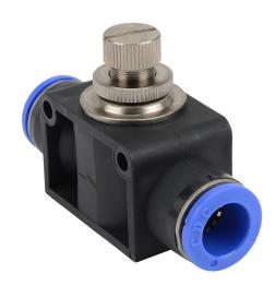
NITRA pneumatic push-to-connect fitting, inline flow control valve, thermoplastic (PBT) body, (1) 12mm push-to-connect to (1) 12mm push-to-connect. Package of 2.
