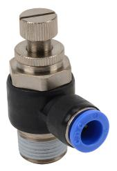
NITRA pneumatic push-to-connect fitting, elbow flow control valve, rotating, meter-out, thermoplastic (PBT) body, nickel-plated brass threads, (1) R3/8 male BSPT to (1) 5/16in (8mm) push-to-connect. Package of 2.
