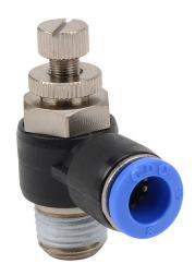
NITRA pneumatic push-to-connect fitting, elbow flow control valve, rotating, meter-out, thermoplastic (PBT) body, nickel-plated brass threads, (1) R1/4 male BSPT to (1) 5/16in (8mm) push-to-connect. Package of 2.
