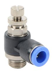
NITRA pneumatic push-to-connect fitting, elbow flow control valve, rotating, meter-out, thermoplastic (PBT) body, nickel-plated brass threads, 5/16in (8mm) tube to G1/4 BSPP connection(s). Package of 2.
