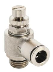
NITRA pneumatic push-to-connect fitting, elbow flow control valve, rotating, meter-out, nickel-plated brass body, nickel-plated brass threads, 5/16in (8mm) push-to-connect to G1/4 BSPP. Package of 2.
