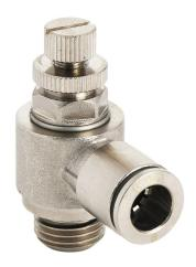
NITRA pneumatic push-to-connect fitting, elbow flow control valve, rotating, meter-out, nickel-plated brass body, nickel-plated brass threads, (1) G1/4 male BSPP to (1) 5/16in (8mm) push-to-connect. Package of 2.
