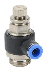
NITRA pneumatic push-to-connect fitting, elbow flow control valve, rotating, meter-out, thermoplastic (PBT) body, nickel-plated brass threads, (1) G1/2 male BSPP to (1) 5/16in (8mm) push-to-connect. Package of 2.
