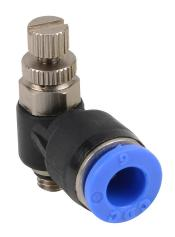
NITRA pneumatic push-to-connect fitting, elbow flow control valve, rotating, meter-out, thermoplastic (PBT) body, nickel-plated brass threads, (1) M5 x 0.8 male ISO to (1) 6mm push-to-connect. Package of 2.
