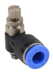
NITRA pneumatic push-to-connect fitting, elbow flow control valve, rotating, meter-out, thermoplastic (PBT) body, nickel-plated brass threads, 6mm tube to M5 X 0.8 threaded connection(s). Package of 2.
