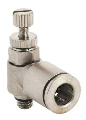
NITRA pneumatic push-to-connect fitting, elbow flow control valve, rotating, meter-out, nickel-plated brass body, nickel-plated brass threads, (1) M5 x 0.8 male ISO to (1) 6mm push-to-connect. Package of 2.
