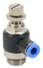
NITRA pneumatic push-to-connect fitting, elbow flow control valve, rotating, meter-out, thermoplastic (PBT) body, nickel-plated brass threads, (1) G3/8 male BSPP to (1) 6mm push-to-connect. Package of 2.
