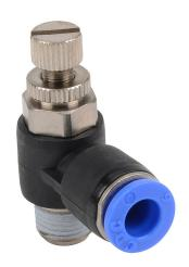
NITRA pneumatic push-to-connect fitting, elbow flow control valve, rotating, meter-out, thermoplastic (PBT) body, nickel-plated brass threads, (1) R1/8 male BSPT to (1) 6mm push-to-connect. Package of 2.
