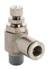
NITRA pneumatic push-to-connect fitting, elbow flow control valve, rotating, meter-out, nickel-plated brass body, nickel-plated brass threads, (1) R1/8 male BSPT to (1) 6mm push-to-connect. Package of 2.
