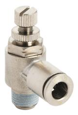
NITRA pneumatic push-to-connect fitting, elbow flow control valve, rotating, meter-out, nickel-plated brass body, nickel-plated brass threads, (1) 1/8in male NPT to (1) 6mm push-to-connect. Package of 2.
