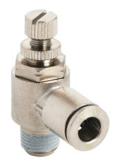
NITRA pneumatic push-to-connect fitting, elbow flow control valve, rotating, meter-out, nickel-plated brass body, nickel-plated brass threads, 6mm push-to-connect to 1/8in NPT. Package of 2.
