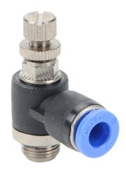
NITRA pneumatic push-to-connect fitting, elbow flow control valve, rotating, meter-out, thermoplastic (PBT) body, nickel-plated brass threads, (1) G1/8 male BSPP to (1) 6mm push-to-connect. Package of 2.
