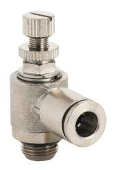
NITRA pneumatic push-to-connect fitting, elbow flow control valve, rotating, meter-out, nickel-plated brass body, nickel-plated brass threads, 6mm push-to-connect to G1/8 BSPP. Package of 2.
