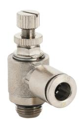
NITRA pneumatic push-to-connect fitting, elbow flow control valve, rotating, meter-out, nickel-plated brass body, nickel-plated brass threads, (1) G1/8 male BSPP to (1) 6mm push-to-connect. Package of 2.
