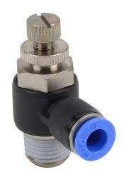
NITRA pneumatic push-to-connect fitting, elbow flow control valve, rotating, meter-out, thermoplastic (PBT) body, nickel-plated brass threads, (1) R1/4 male BSPT to (1) 6mm push-to-connect. Package of 2.
