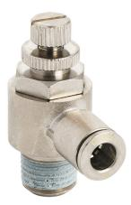
NITRA pneumatic push-to-connect fitting, elbow flow control valve, rotating, meter-out, nickel-plated brass body, nickel-plated brass threads, (1) R1/4 male BSPT to (1) 6mm push-to-connect. Package of 2.
