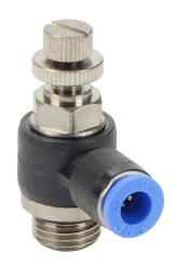
NITRA pneumatic push-to-connect fitting, elbow flow control valve, rotating, meter-out, thermoplastic (PBT) body, nickel-plated brass threads, 6mm tube to G1/4 BSPP connection(s). Package of 2.
