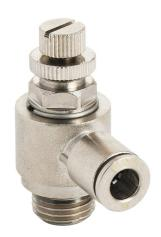
NITRA pneumatic push-to-connect fitting, elbow flow control valve, rotating, meter-out, nickel-plated brass body, nickel-plated brass threads, (1) G1/4 male BSPP to (1) 6mm push-to-connect. Package of 2.
