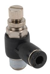
NITRA pneumatic push-to-connect fitting, elbow flow control valve, rotating, meter-out, thermoplastic (PBT) body, nickel-plated brass threads, 5/32in (4mm) tube to 1/8in NPT connection(s). Package of 2.
