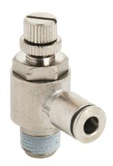
NITRA pneumatic push-to-connect fitting, elbow flow control valve, rotating, meter-out, nickel-plated brass body, nickel-plated brass threads, (1) 1/8in male NPT to (1) 5/32in (4mm) push-to-connect. Package of 2.
