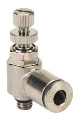
NITRA pneumatic push-to-connect fitting, elbow flow control valve, rotating, meter-out, nickel-plated brass body, nickel-plated brass threads, (1) #10-32 male UNF to (1) 5/32in (4mm) push-to-connect. Package of 2.
