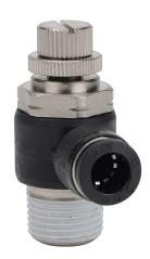
NITRA pneumatic push-to-connect fitting, elbow flow control valve, rotating, meter-out, thermoplastic (PBT) body, nickel-plated brass threads, (1) 3/8in male NPT to (1) 5/16in (8mm) push-to-connect. Package of 2.
