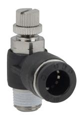
NITRA pneumatic push-to-connect fitting, elbow flow control valve, rotating, meter-out, thermoplastic (PBT) body, nickel-plated brass threads, (1) 1/8in male NPT to (1) 5/16in (8mm) push-to-connect. Package of 2.
