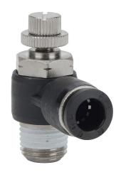
NITRA pneumatic push-to-connect fitting, elbow flow control valve, rotating, meter-out, thermoplastic (PBT) body, nickel-plated brass threads, (1) 1/4in male NPT to (1) 5/16in (8mm) push-to-connect. Package of 2.
