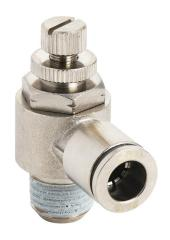
NITRA pneumatic push-to-connect fitting, elbow flow control valve, rotating, meter-out, nickel-plated brass body, nickel-plated brass threads, (1) 1/4in male NPT to (1) 5/16in (8mm) push-to-connect. Package of 2.
