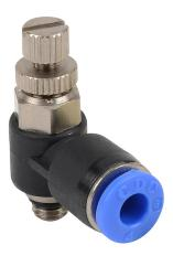
NITRA pneumatic push-to-connect fitting, elbow flow control valve, rotating, meter-out, thermoplastic (PBT) body, nickel-plated brass threads, (1) M5 x 0.8 male ISO to (1) 5/32in (4mm) push-to-connect. Package of 2.
