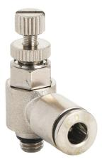
NITRA pneumatic push-to-connect fitting, elbow flow control valve, rotating, meter-out, nickel-plated brass body, nickel-plated brass threads, (1) M5 x 0.8 male ISO to (1) 5/32in (4mm) push-to-connect. Package of 2.
