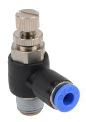
NITRA pneumatic push-to-connect fitting, elbow flow control valve, rotating, meter-out, thermoplastic (PBT) body, nickel-plated brass threads, (1) R1/8 male BSPT to (1) 5/32in (4mm) push-to-connect. Package of 2.
