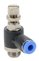
NITRA pneumatic push-to-connect fitting, elbow flow control valve, rotating, meter-out, thermoplastic (PBT) body, nickel-plated brass threads, (1) G1/8 male BSPP to (1) 5/32in (4mm) push-to-connect. Package of 2.
