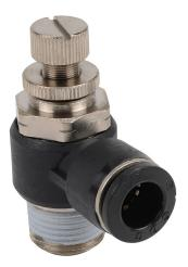
NITRA pneumatic push-to-connect fitting, elbow flow control valve, rotating, meter-out, thermoplastic (PBT) body, nickel-plated brass threads, (1) 3/8in male NPT to (1) 3/8in push-to-connect. Package of 2.
