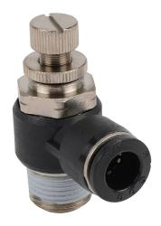
NITRA pneumatic push-to-connect fitting, elbow flow control valve, rotating, meter-out, thermoplastic (PBT) body, nickel-plated brass threads, 3/8in tube to 3/8in NPT connection(s). Package of 2.
