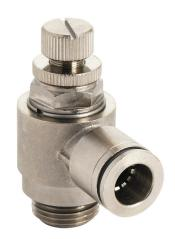
NITRA pneumatic push-to-connect fitting, elbow flow control valve, rotating, meter-out, nickel-plated brass body, nickel-plated brass threads, (1) G3/8 male BSPP to (1) 3/8in push-to-connect. Package of 2.
