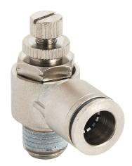
NITRA pneumatic push-to-connect fitting, elbow flow control valve, rotating, meter-out, nickel-plated brass body, nickel-plated brass threads, (1) 1/4in male NPT to (1) 3/8in push-to-connect. Package of 2.
