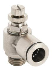
NITRA pneumatic push-to-connect fitting, elbow flow control valve, rotating, meter-out, nickel-plated brass body, nickel-plated brass threads, (1) G1/4 male BSPP to (1) 3/8in push-to-connect. Package of 2.
