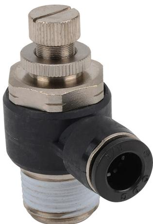
NITRA pneumatic push-to-connect fitting, elbow flow control valve, rotating, meter-out, thermoplastic (PBT) body, nickel-plated brass threads, (1) 1/2in male NPT to (1) 3/8in push-to-connect. Package of 2.
