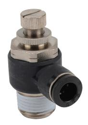
NITRA pneumatic push-to-connect fitting, elbow flow control valve, rotating, meter-out, thermoplastic (PBT) body, nickel-plated brass threads, (1) 1/2in male NPT to (1) 3/8in push-to-connect. Package of 2.
